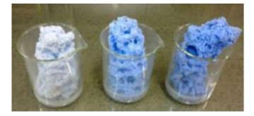
Pigments CB1, CB2, CB3 with foamed structure after SCS in the system Al-Co-Ba-Mg-O (81,5%  $Al(NO_3)_3+10,73\%+Ba(NO_3)_2,77\%$   $Mg(NO_3)_2+XCo(NO_3)_2+60\%$  urea).
