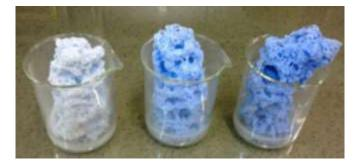
Pigments CB1, CB2, CB3 with foamed structure after SCS in the system Al-Co-Ba-Mg-O (81,5%  $Al(NO_3)_3+10,73\%+Ba(NO_3)_2,77\%$   $Mg(NO_3)_2+XCo(NO_3)_2+60\%$  urea).
